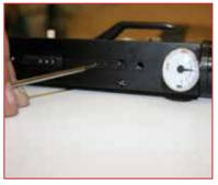
**adjust, as this may cause the gun to fire prematurely or not operate correctly and make the rifle unsafe**. Always check your settings to ensure correct and safe operation of the rifle. Always ensure that operation of the safety is unaffected by any alterations you may make to the trigger mechanism.
