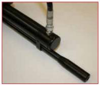
2) When charging is complete, bleed the excess air using the fill apparatus bleed screw and remove the fill adapter from the rifle. When finished, rotate the protective cover to prevent contamination of the fill port.
