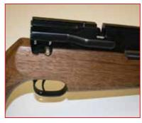
In addition to the safety catch, a loaded and cocked rifle can be made safe by decocking (uncocking). To decock the rifle, first pull the sidelever back to the rear position and remove the magazine. While holding the sidelever, squeeze the trigger and let the lever return forward under your control. The rifle is now decocked.
